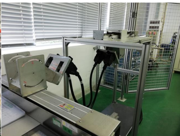
Custom X-Y movement tester for a railway jumper cable
