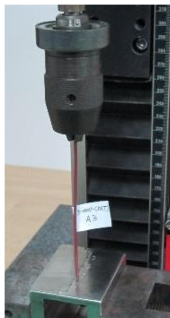
Mating cycle test with insertion and withdrawal force profile of a HARTING D-Sub male and female connector
