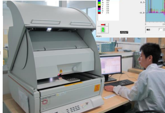
Energy dispersive X-ray analysis (RFA) with energy spectrum
