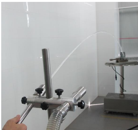
IPX5 hose-proof test on a Han® 16B housing
