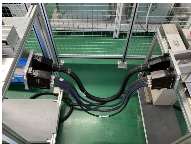
Custom X-Y movement tester for a railway jumper cable
