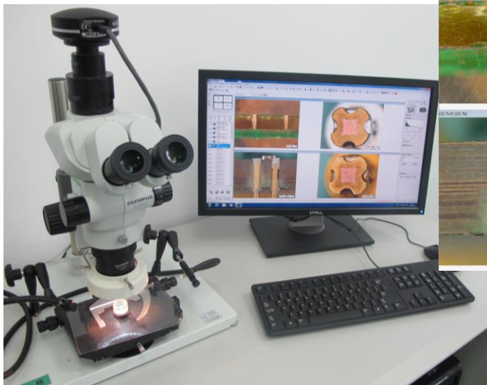
Microscopic examination on the grinded cross section of a multi- layer backplane soldering hole and a crimping connection
