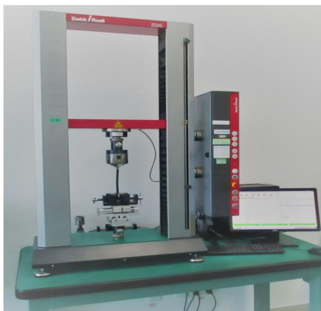
Insertion and withdrawal force performance of a HARTING vehicle connector after 10000 cycles durability test
