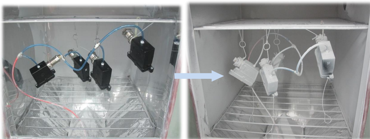
IP6X dust test arrangement on a Han® Hood/Cable gland assembly
