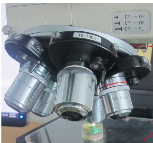
Microscopic examination on a grinded & polished cross section of a through hole layer
