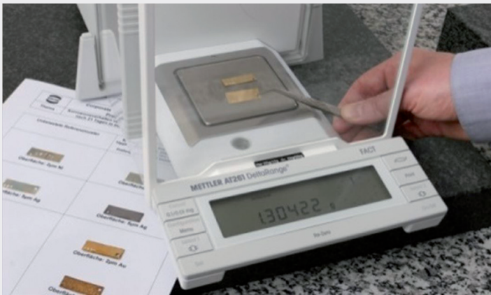
Weighing of galvanically coated testing plates before and after the flowing mixed gas corrosion test
