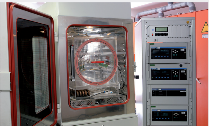
Flowing mixed gas corrosion test with analytics
