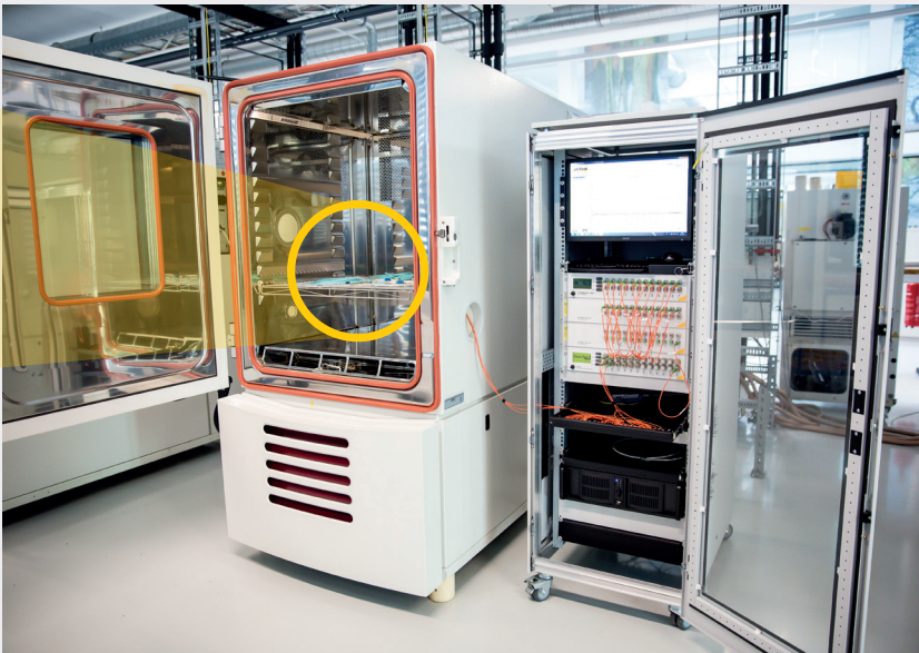
Recording the change in attenuation and return loss under climatic and mechanical stress
