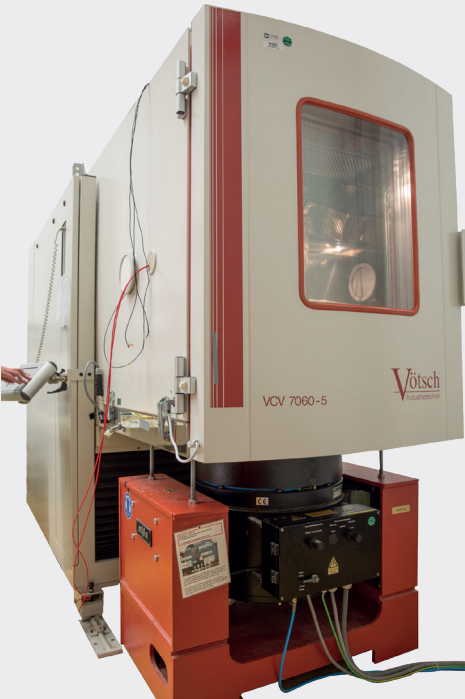
Vibration test with climatic overlay and current load
