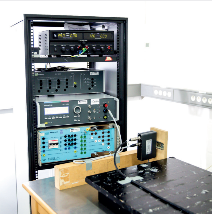
Examination of the interference immunity against high energetic, transient interference pulses (Surge)
