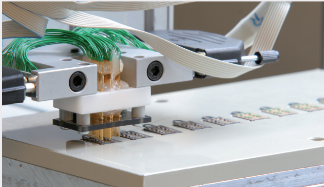
Measuring adapter for automated resistance measurements (resistance, insulating resistance)
