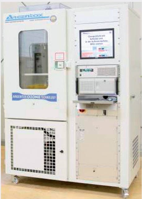
Ozone test chamber: application in the aging and testing of material
