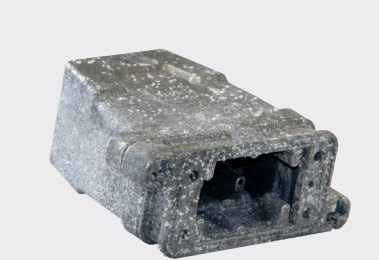
Influence of salt mist on a test object (alloy of die-cast aluminum) without corrosion-resistant surface
